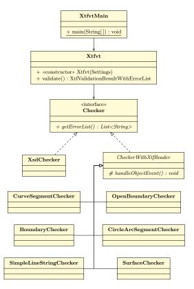
Figure 1: Class diagram of important classes in xtfvt.
